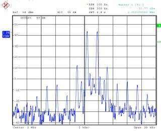
Tx: 14.5MHz Carrier Suppression= 49.24dBm-(-13.48dBm)=62.72dB Limit: >40dB
